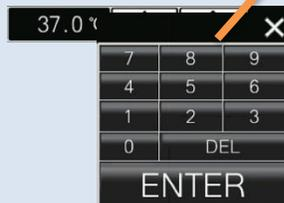
**Number Pad:** Tap the current setpoint value. The number pad opens. Input the desired setpoint and press Enter on the keypad to set.
