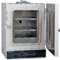
The BACTRON400HP requires a scrubber cartridge oven to reactivate the O<sub>2</sub>/activated carbon media scrubber cartridges.
