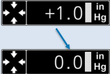
**Zero the Pressure Displays** This sets the pressure gauges to local conditions. See page 48.
