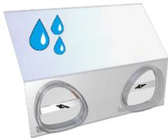
Fogging and Humidity. Mild or heavy condensation may take place inside the chamber during the cycle. This is due in part to the formation of water vapor as the catalytic O<sub>2</sub> scrubber removes large amounts of oxygen. High ambient humidity and cool room temperatures also contribute. The condensate should dissipate by the end of the cycle as oxygen decreases and as the condensate controller removes water vapor from the chamber atmosphere.
