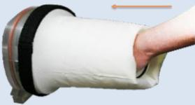
Push on the ballooned sleeve while watching the manometer to see if the water level changes.
